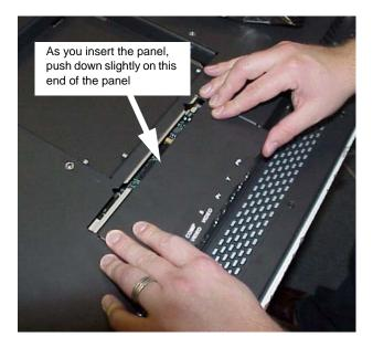
10. Secure the DVI or SDI replacement cover panel using the screws you removed earlier.
